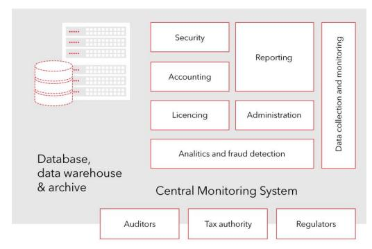
Figure 1: Central Monitoring System modules
